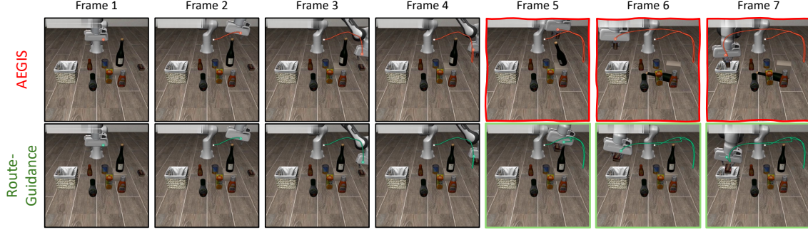
Fig. 2: Qualitative comparison on SafeLIBERO. Task: pick up the chocolate pudding and place it in the basket. Top row: AEGIS (Success, Collision). Bottom row: Ours (Success, Collision-free).
